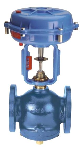
The rugged Powers Flowrite II Type SI balanced (single seat iron body) control valve is primarily used for steam and water modulating applications with moderate pressure drops. The SI value is available with the Powers 46  $in^2$  and 100  $in^2$ actuators. Actuator selection depends on valve size and flowing system pressure drop across the valve.
