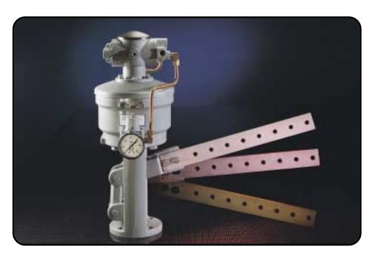
Conoflow's Pneumatic Lever Actuators are rugged and powerful units used to automatically position dampers, louvers, variable pitch fans and to make various mechanical adjustments to process machinery. Low profile (only 18" high) requires less headroom. A sturdy ductile iron yoke with large mounting base provides rigid mounting. The steel lever arm has eight take-off positions for stroke flexibility.
